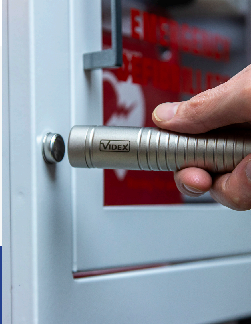
Above: Technician records the date and time of the yearly test of emergency equipment by scanning an iButton with PulseStar.
