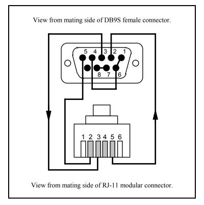
Figure C-4 9-Pin Serial Port Cable Configuration
