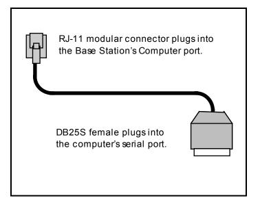
Figure C-1 25-Pin Serial Port Cable
