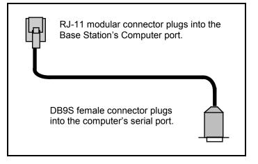
Figure C-3 9-Pin Serial Port Cable
