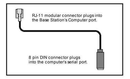
Figure C-5 DIN 8 Serial Port Cable
