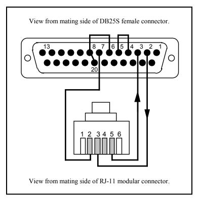
Figure C-2 25-Pin Serial Port Cable Configuration
