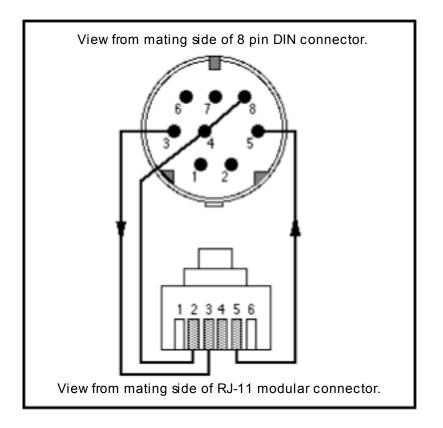
Figure C-6 DIN 8 Serial Port Cable Pin Configuration
