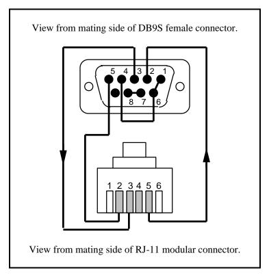
Figure D-4 9-Pin Serial Port Cable Configuration
