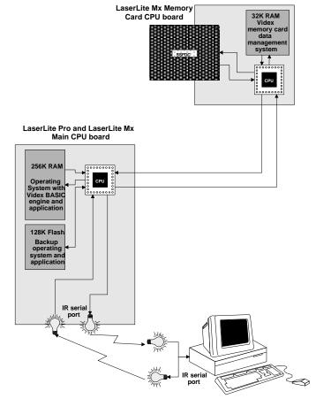
Figure 1-4 LaserLite Pro and LaserLite Mx System Components
