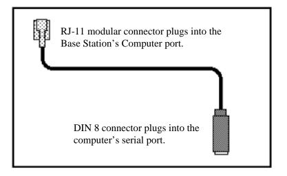
Figure D-5 DIN 8 Serial Port Cable
