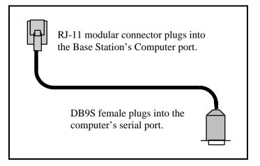
Figure D-3 9-Pin Serial Port Cable
