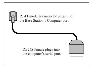
Figure D-1 25-Pin Serial Port Cable
