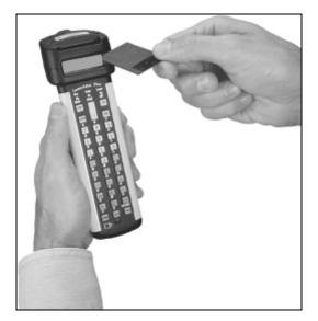
Figure 2-2 Installing Memory Card
