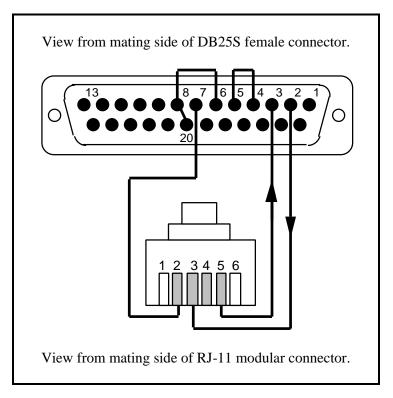
Figure D-2 25-Pin Serial Port Cable Configuration
