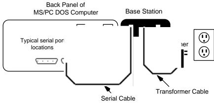
Figure 1-12 Base Station Connections
